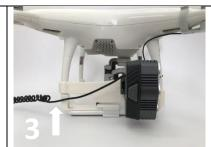
IMPORTANT: Route the spiral wire BEHIND the REAR RIGHT and REAR LEFT landing gear
