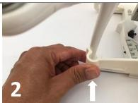
Slide the **REAR SIDE** of the LED bracket over the **REAR RIGHT** landing gear until it locks in place
